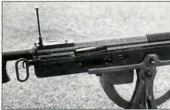
The cocking handle on the U.S. Navy Mark V Model 1917 machine gun is that of the Marlin-Rockwell aircraft guns.
